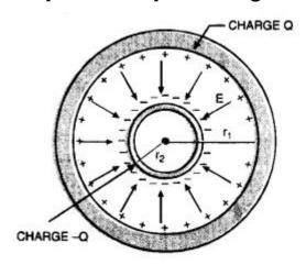
$$C = \frac{4\pi\varepsilon_0 r_1 r_2}{r_1 - r_2}$$
