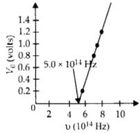
The first four spots on the V0 versus n plot are almost exactly on a straight line that crosses the x-axis at the threshold frequency, u0 = 5.0 1014 Hz. Since u u0 corresponds to the fifth point (u = 4.3 1014 Hz), there is no photoelectric emission and no stopping voltage is needed to stop the current.
