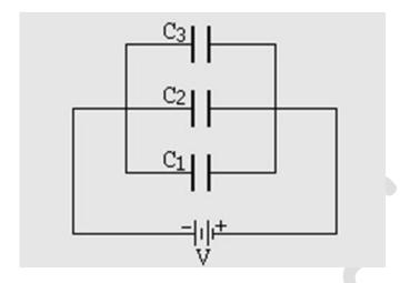
The equivalent capacitance is given by
