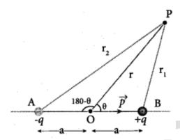
Electrostatic potential due to an electric dipole at any point P inclined at an angle  $\theta$  whose position vector is r w.r.t mid point of the dipole is given by;
